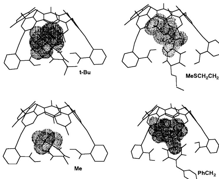
Fig. 2. The calculated structures of the complexes. Van der Waals surface of the inner substituents is represented as dot surface
